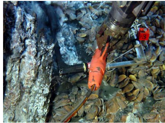
Fig. 3. In situ analysis using Alchemist manipulated by the ROV Victor, Atos cruise 2001, Lucky Strike. Photo © IFREMER
