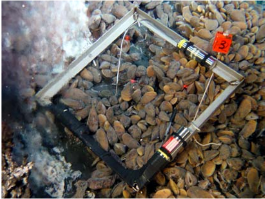
Fig. 4. Monitoring of temperature over a clump of mussels, ATOS cruise 2001, Lucky Strike. Photo © IFREMER
